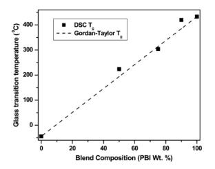
Figure 10: Variation of the glass transition temperature (Tg) of PBI as a function of PBI/PVDF blend composition. The solid points are the experimentally obtained Tg values from the DSC study, and the dotted line is the calculated Tg curve according to the Gordon-Taylor equation with k=1 (reproduced with permission from the Amer. Chem. Soc.; Arunbabu, D.; Sannigrahi, A.; Jana, T; *J. Phys. Chem. B* **2008**, *112*, 5305).
