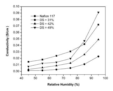
Figure 33: Proton conductivity *versus* the relative humidity of PSSA-*b*-PVDF-*b*-PSSA triblock copolymers and Nafion® 117 membranes; DS stands for degree of sulfonation (reproduced with permission from the Amer. Chem. Soc, Xu *et al.; Chem. Mater.*, **2007**, *19*, 5937<sup>336</sup>).
