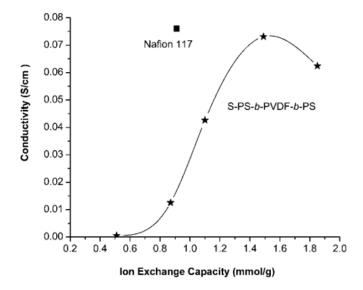
Figure 32: Conductivities of Nafion® 117 and of membranes achieved from PSSA-b-PVDFb-PSSA triblock copolymer as a function of the ion-exchange capacity (reproduced with permission from the Amer. Chem. Soc, *Chem. Mater.*, **2007**, *19*, 5937; Xu *et al.*<sup>336</sup>)
