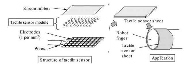
Figure 11: Tactile sensor for robotic applications (reproduced with permission from K. Takashima *et al.*, *Sensors and Actuators*, **2008**, *A 144*, *90*).
