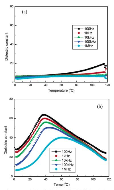
Figure 13: Dielectric constant of (a) poly(VDF-co-CTFE) (92/8 mol %) copolymer (melting temperature,  $T_m$ = 145.0 °C; Curie temperature,  $T_c$ = non-assessed) and (b) poly(VDF-ter-TrFE-ter-CTFE) (65.6/26.7/7.7 mol %) terpolymer ( $T_m$ = 123.6 °C and  $T_c$ = 23.8 °C) (reproduced with permission from the *Amer. Chem. Soc.* Zhang, Z.; Mike Chung T.C.; *Macromolecules*, **2007**, *40*, 783<sup>128</sup>).
