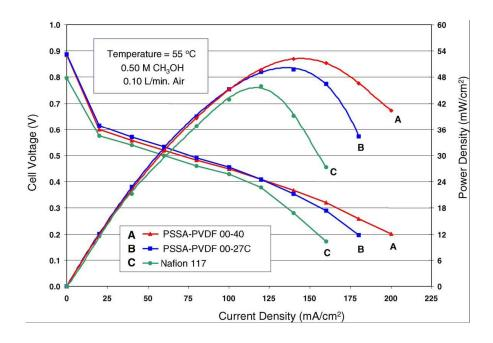
Figure 8: Polarization curve of PVDF/PSSA membrane achieved from semi interpenetrated polymer network (reproduced with permission from Elsevier; Prakash, G.K.S. *et al.*; *J. Fluorine Chem.* **2004**, *125*, 1217<sup>98</sup>).
