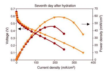
Figure 18: Polarization curves of: coated Nafion<sup>®</sup> (orange) and virgen Nafion<sup>®</sup> 117 (brown) at 30 °C (reproduced with permission from Elsevier; Cho et al.; *J. Power Sources*, **2006**, 159, 524).
