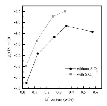
Figure 21: The Li+ content of gel polymer electrolyte without  $SiO_2$  (-O-) and with  $SiO_2$  (-square-) dependence on the ionic conductivity (reproduced with permission from the *Amer*. *Chem. Soc.* (Wang et al. *J. Phys. Chem. B* **2004**, *108*, 1365<sup>182</sup>)).
