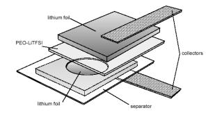
Figure 3: Lithium battery sketch (reproduced with permission from the American Chemical Society; Bouchet, R.; Lascaud, S.; Rosso, M.; *J. Electrochem. Soc.*, **2003**, *150*, A1385).
