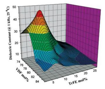
Figure 15: A three-dimensional plot of room temperature dielectric constants at 1 kHz for the P(VDF-CTFE-TrFE) terpolymers (reproduced with permission from the Amer. Chem. Soc. Lu, Y.; Claude, J.; Neese, B.; Zhang, Q.M.; Wang, Q.; *J. Amer. Chem. Soc.*, **2006**, *128*, 8120<sup>126a</sup>).
