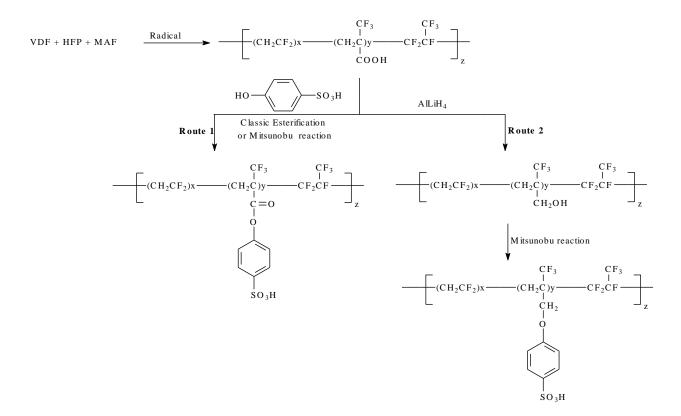
Scheme 59: Obtaining of original fuel cell membranes from poly(VDF-ter-HFP-ter-MAF) terpolymers (where MAF stands for  $\alpha$ -trifluoromethacrylic acid)<sup>380</sup>
