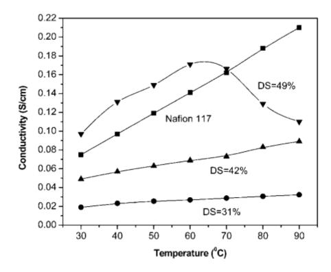
Figure 34: Variation of proton conductivity measured under 95 % relative humidity *versus* temperature for PSSA-*b*-PVDF-*b*-PSSA triblock copolymers and Nafion®117 membranes (reproduced with permission from the Amer. Chem. Soc, Xu *et al.; Chem. Mater.*, **2007**, *19*, 5937<sup>336</sup>).
