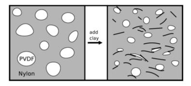
Figure 5: Cartoon showing the effect of the clay in PVDF/nylon-6 blends by melt compounding<sup>90</sup> (reproduced with permission from *Amer. Chem. Soc.*, Fluoropolymer Conference 2008, Charleston, Oct. 19-22, 2008)
