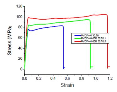
Figure 4: Tensile stress/strain curves for PVDF/nylon-6 blends with various contents of organoclays<sup>90</sup> (reproduced with permission from *Amer. Chem. Soc.*, Fluoropolymer Conference 2008, Charleston, Oct. 19-22, 2008)
