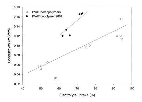
Figure 20: Conductivity as a function of the electrolyte uptake for low-porous PVDF and poly(VDF-co-HFP) copolymers (PVDF copolymer 2801) membranes (reproduced with permission from Elseveir; Michot, T.; Nishimoto, A.; Watanabe, M.; *Electrochim. Acta*, **2000**, *45*, 1347<sup>170b</sup>).
