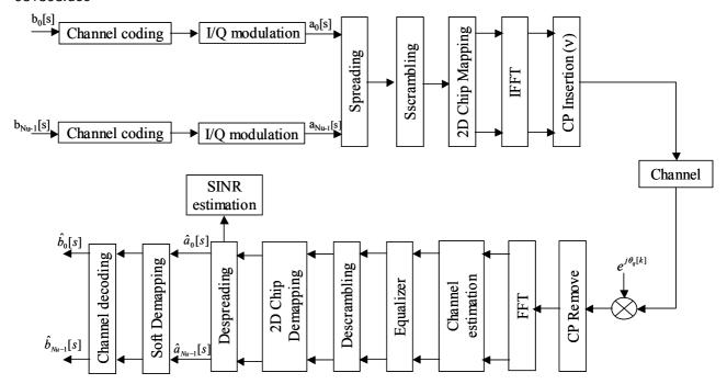
Figure 1- OFDM-CDMA Transceiver.
