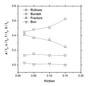
Fig. 16 – Friction effects on the characteristic features of sheared edge predicted by FE simulations.
