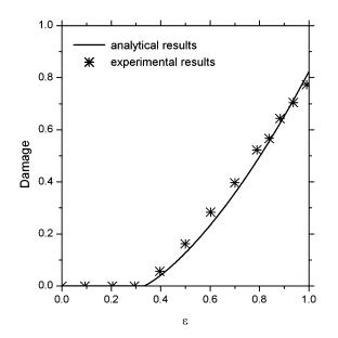
Fig. 3 – Comparison between the damage evolution predicted with Eq. (7) and the experimental results obtained by (Dufailly, 1980) for  $\dot{e} = 0.004 \text{ s}^{-1}$  and T = 298 K.
