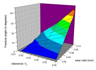
Fig. 15 – Effect of tool wear on fracture angle for a blanking clearance ranged between 15  $\mu$ m and 60  $\mu$ m.
