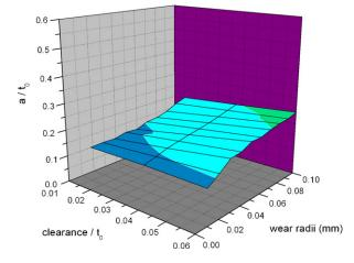
Fig. 11 – Effect of tool wear on rollover depth for a blanking clearance ranged between 15  $\mu$ m and 60  $\mu$ m.
