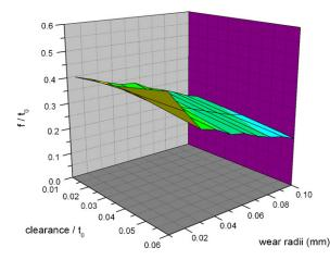
Fig. 13 – Effect of tool wear on fracture depth for a blanking clearance ranged between 15  $\mu$ m and 60  $\mu$ m.
