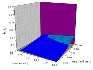
Fig. 14 – Effect of tool wear on burr height for a blanking clearance ranged between 15  $\mu m$  and 60  $\mu m.$
