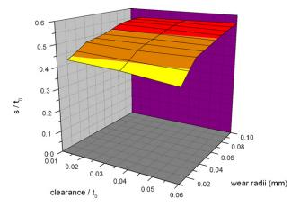
Fig. 12 – Effect of tool wear on burnish depth for a blanking clearance ranged between 15  $\mu m$  and 60  $\mu m.$
