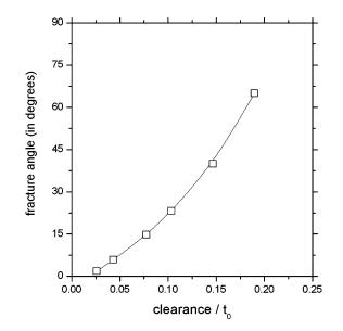
Fig. 8 – Fracture angle evolution predicted by FE simulations as a function of blanking clearance.
