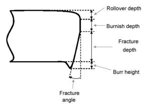
Fig. 1 - Characteristic features of a sheared edge.
