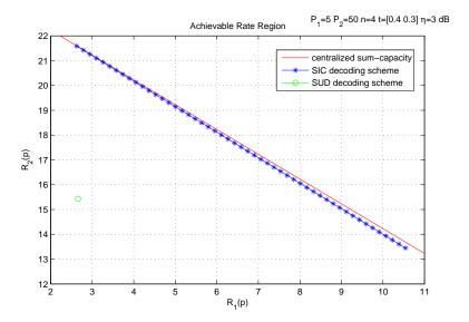
Fig. 4. Spatial PA game. Achievable rate region for  $P_1 = 5$ ,  $P_2 = 50$ ,  $n_r = n_t = 4$ ,  $\eta = 3$  dB,  $t_1 = 0.4$ ,  $t_2 = 0.3$ . By varying p allows to move along a segment close to the centralized sum-capacity, similar to the SISO MAC channels.
