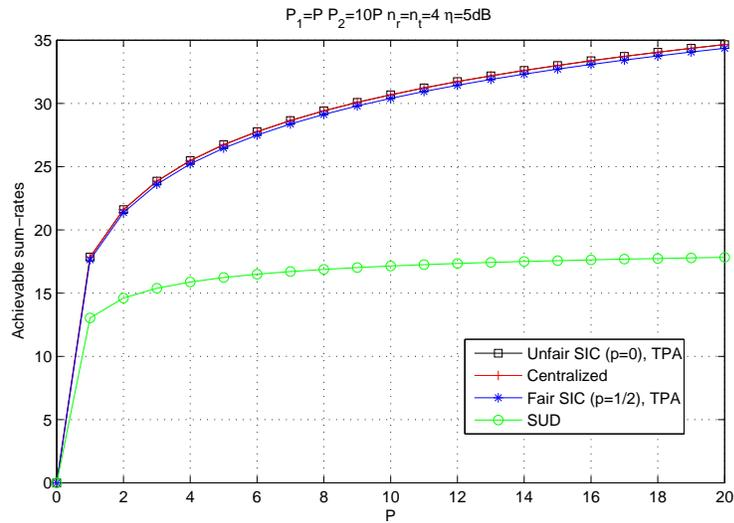
Fig. 2. Temporal PA game. MAC sum-rate versus the transmit power  $P$  for  $P_1 = P, P_2 = 10P, n_r = n_t = 4, \eta = 5$  dB. Comparison between the fair SIC decoding scheme ( $p = \frac{1}{2}$ ), the unfair SIC scheme ( $p = 0$ ), and SUD decoding scheme.
