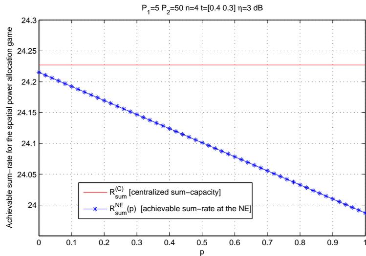
Fig. 3. Spatial PA game. MAC sum-rate versus  $p$  for  $P_1 = 5, P_2 = 50, n_r = n_t = 4, \eta = 3$  dB,  $t_1 = 0.4, t_2 = 0.3$ . The achievable network sum-rate of fading MIMO MACs is linear w.r.t.  $p \in [0, 1]$  and is very close to the centralized upper bound. The optimal distribution obtained with the Stackelberg game is  $p^* = 0$ .
