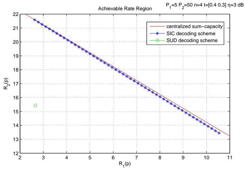
Fig. 4. Spatial PA game. Achievable rate region for  $P_1 = 5$ ,  $P_2 = 50$ ,  $n_r = n_t = 4$ ,  $\eta = 3$  dB,  $t_1 = 0.4$ ,  $t_2 = 0.3$ . By varying  $p$  allows to move along a segment close to the centralized sum-capacity, similar to the SISO MAC channels.
