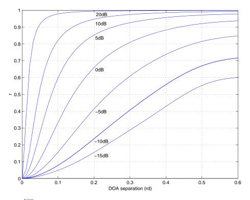
Fig.5 Ratio  $r \stackrel{\text{def}}{=} \frac{\text{CRB}_{\text{NU}}^{\text{NCG}}(\theta_1)}{\text{CRB}_{\text{NU}}^{\text{CG}}(\theta_1)}$  as a function of the DOA separation for different values of SNR with  $\rho_2 = \rho_1 = 1$  and  $\Delta \phi = 0.52 nd$
