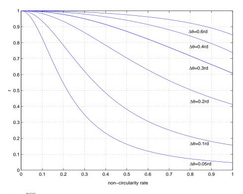
Fig.4 Ratio  $r \stackrel{\text{def}}{=} \frac{\text{CRB}_{\text{NU}}^{\text{NCG}}(\theta_1)}{\text{CRB}_{\text{NU}}^{\text{CG}}(\theta_1)}$  as a function of the non-circularity rate for different values of DOA separation with SNR = -5dB and  $\Delta \phi = 0.52rd$ .
