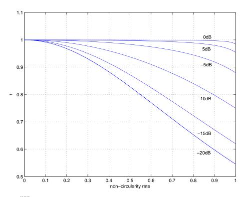
Fig.3 Ratio  $r \stackrel{\text{def}}{=} \frac{\text{CRB}_{\text{NU}}^{\text{NCG}}(\theta_1)}{\text{CRB}_{\text{NU}}^{\text{CG}}(\theta_1)}$  as a function of the non-circularity rate  $\rho_1$  for different values of the SNR.
