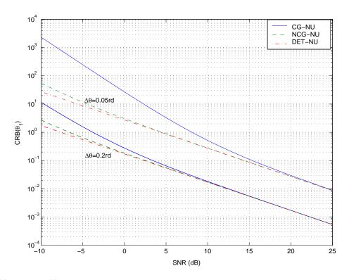
Fig.2  $CRB_{NU}^{NCG}(\theta_1)$ ,  $CRB_{NU}^{CG}(\theta_1)$  and  $CRB_{NU}^{DET}(\theta_1)$  as a function of the SNR for two values of the DOA separation with  $\Delta \phi = 0.52rd$ .
