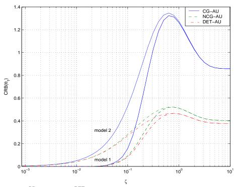
Fig.1 CRB<sup>NCG</sup><sub>AU</sub>( $\theta_1$ ), CRB<sup>CG</sup><sub>AU</sub>( $\theta_1$ ) and CRB<sup>DET</sup><sub>AU</sub>( $\theta_1$ ) as a function of  $\zeta$  for the first and second models with  $\Delta \theta = 0.1 rd$ , SNR= 0dB and  $\Delta \phi = 0.52 rd$ .
