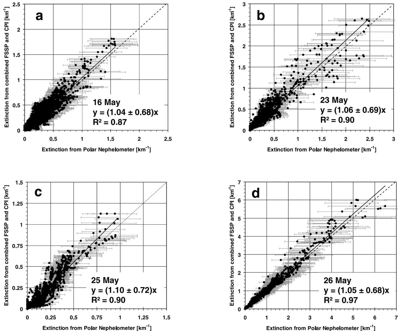
**Figure 7.** Comparison between extinction coefficients from combined FSSP-300 and CPI instruments and Polar Nephelometer probe for the (a) 16, (b) 23, (c) 25, and (d) 26 May situations. The slope parameters with their uncertainties and correlation coefficients are reported. Horizontal gray bars represent the 25% uncertainties on Polar Nephelometer measurements.
