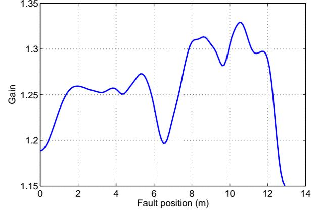
Fig. 6. The values of  $G(Z_F)$  in terms of the fault's position. The studied system is represented in Figure 2. The fault is being moved from the 140  $\Omega$  impedance towards the 200  $\Omega$  impedance.
