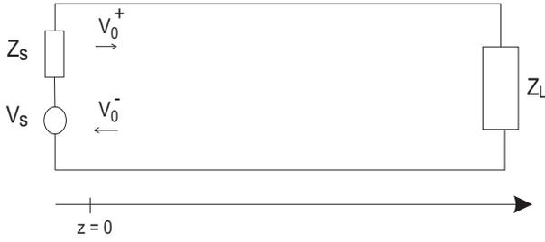
Fig. 3. A model illustrating the transmission line theory used in the paper:  $V_0^+$  and  $V_0^-$  are the modal variables to be determined in order to characterize the voltage and current propagation along the line.
