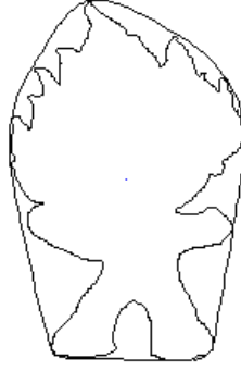
Figure 6: Illustration of convex hull
