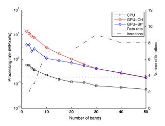
**Fig. 7** Anomaly detection processing rate for different choices of number of bands. The *solid lines* show the processing rate for the different implementations, while the *dotted line* shows the sensor data rate (see the left *y*-axis). The *dash-dot line* shows the number of iterations needed to reach convergence for the different band counts (see the right *y*-axis)
