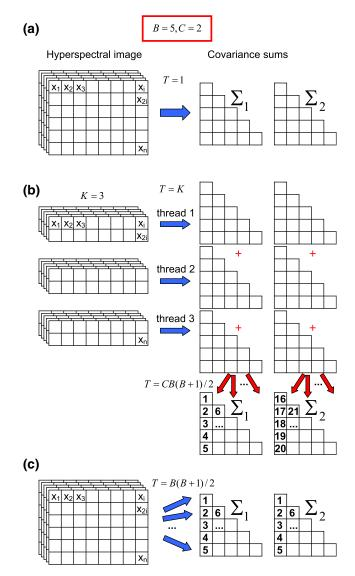
**Fig. 3** Different approaches for calculation of the covariance sums: **a** sequential algorithm; **b** parallel algorithm—chunking approach; **c** parallel algorithm—spectral-level parallelism. The figure assumes B=5, C=2 and K=3. The *numbers* in the covariance sums' matrix cells correspond to different parallel threads
