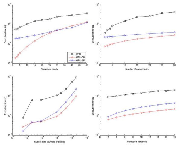
**Fig. 5** Total execution time for the three implementations when varying different parameters. The plots show the execution time for different choices of number of bands (*top left*), number of components
