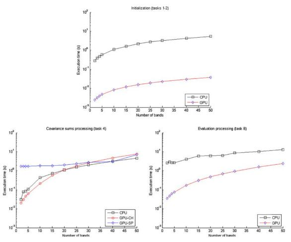
**Fig. 6** Execution time for important parts of the implementations. The *plots* show the difference between the implementations in execution time for the initialization tasks (*top*), the covariance sums processing task (*bottom left*) and the evaluation processing task
