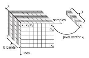
Fig. 1 Structure of the hyperspectral image data
