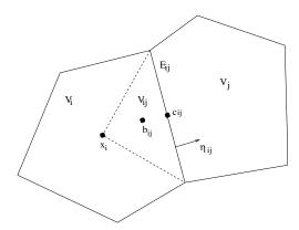
Fig. 2. Finite volume mesh
