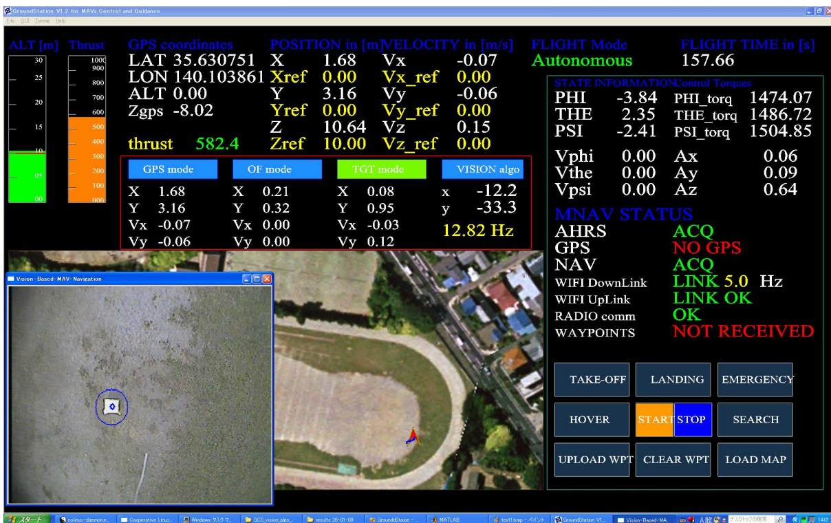
Fig. 5 The interactive interface of the ground control station during vision-based autonomous hovering.
