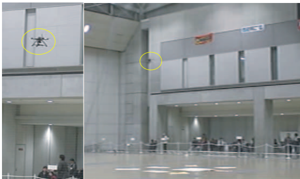
Fig. 8 Indoor fully autonomous flight using optic flow. Demonstration at Tokyo Big Sight for an international exhibition.
