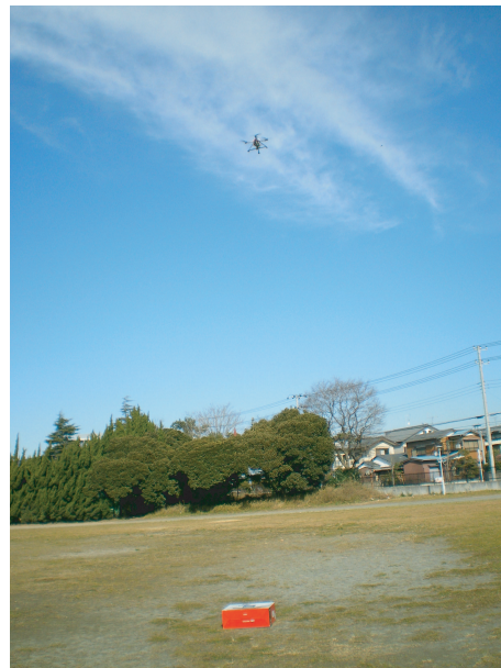
Fig. 10 Rotorcraft during vision-based autonomous hovering above a stationary target.
