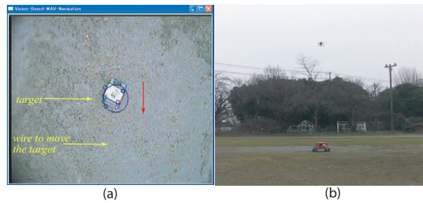
Fig. 13 (a) onboard image showing the detection and tracking of a moving target; (b) MAV tracking the moving target.
