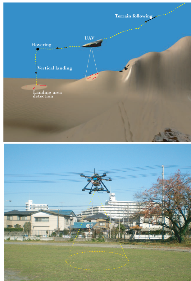
Fig. 1 Visual navigation and control of small rotorcraft UAVs using vision.
