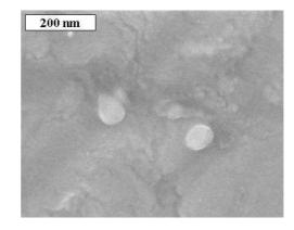
Figure 5: Nanocrystals of 40 nm in radius obtained at  $T = -40^{\circ}C$
