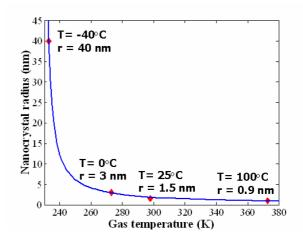
Figure 4: Nanocrystal radius versus gas temperature
