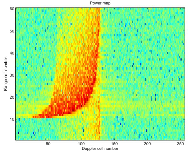
Fig. 3. Power map vs range and Doppler cell.
