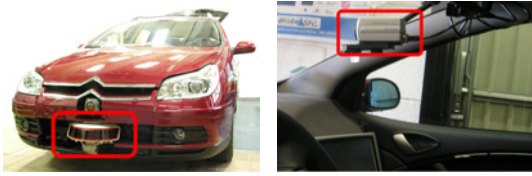
Fig. 6. Experimental platform: Lidar (left), Camera (right)
