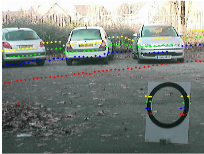
Fig. 7. Projection image of lidar data
