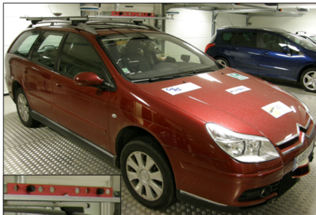
Figure 1. The stereo vision system installed on board the experimental vehicle. In the left-down section, a zoomed view of the stereo vision system
