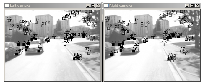
Figure 8. Features points during real-time odometry estimation, \blacksquare : Outliers \square : Inliers
