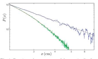
Fig. 2. Experimental measurements of the step size distribution function (log-log scale) in the configuration of Figure 1(a) and (b). With an incident laser beam (green crosses), the observed decay is well fitted by an exponential (red dotted line) as expected from Beer-Lambert law. In the two-cell configuration, the data (continuous blue line) are well fitted by a power law (black dotted line)  $P(x) = 1/x^{\alpha}$ , with  $\alpha = 2.41 \pm 0.12$ .
