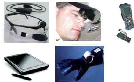
Figure 2. Goggles with integrated screen, See-Through goggles, TabletPC, RFID reader and Data glove
