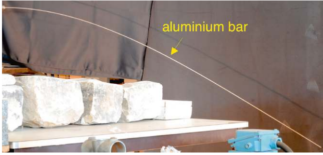
Fig. 12. (Color online) Aluminium bar bending under its own weight.
