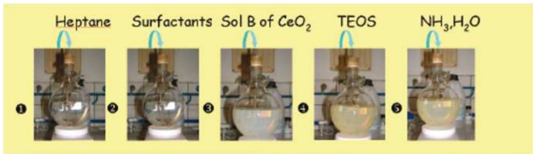
Fig. 1. Five-steps colloid-in oil microemulsion.
