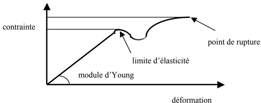
Figure 1. Contrainte = f(déformation).
