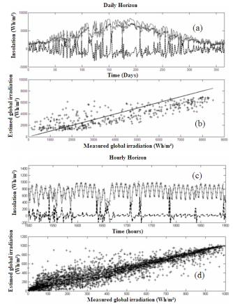
**Figure 1:** Example of simulated and experimental global solar irradiation in Bastia for the daily horizon (a) and in Corte for the hourly horizon (c). Dashed line is the error, solid line is the measured insolation and marks are the prediction. On the bottom corresponds to the correlation between experimental and simulated global irradiation in Bastia for the daily horizon (b) and in Corte for the hourly horizon (d).
