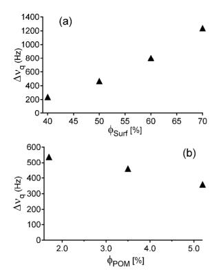
Figure 4: Quadrupolar splitting  $(\Delta v_q)$  of aligned lamellar phases (a) as a function of  $\phi_{Surf}$  at  $\phi_{POM} = 3.5\%$ , and (b) as a function of  $\phi_{POM}$  at  $\phi_{Surf} = 50\%$ . (All measurements were performed at 310K.)
