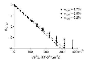
Figure 8: <sup>1</sup>H PGSE-NMR signal decays for samples with constant  $\phi_{Surf} = 50\%$  and varying  $\phi_{POM}$ . As expected, the self-diffusion coefficient of water does not change when the lamellar periodicity of the phase remains constant.
