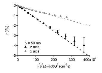
Figure 6: <sup>1</sup>H PGSE-NMR water-signal decays of an aligned sample with  $\phi_{Surf} = 50\%$  and  $\phi_{POM} = 3.5\%$ . The black triangles correspond to a gradient along the z-axis direction, and the grey triangles along the x- or y-axis directions (Diffusion time  $\Delta = 50$  ms). The diffusion anisotropy is clearly demonstrated by the change of gradient. The dotted lines are linear fits to the data using the Stejskal-Tanner equation (1).
