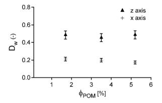
Figure 10: Variation of normalized water self-diffusion coefficients of aligned POM-doped lamellar phases with  $\phi_{POM}$ , at constant  $\phi_{Surf} = 50\%$ . The POM volume fraction does not affect water diffusion.
