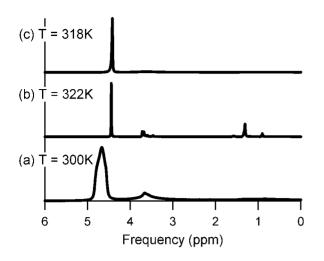
Figure 5: <sup>1</sup>H NMR spectra of a doped  $L_{\alpha}$  phase at different temperatures. (a) Powder-like  $L_{\alpha}$  phase. (b) Isotropic phase at high temperature. The water, ether, and alkyl peaks (located around 4.5, 3.5, and 1.5 ppm, respectively) are well resolved because of the high mobility of the phase. (c) Aligned  $L_{\alpha}$  phase.
