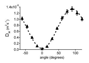
Figure 11: Angular dependence of the water diffusion coefficients in a single-domain of POMdoped L<sub> $\alpha$ </sub> phase ( $\phi_{Surf} = 50\%$ ,  $\phi_{POM} = 3.5\%$ ). The line is a fit to the data using equation (2). The minimum corresponds to  $D_{I/}$  and the maximum to  $D_{\perp}$ .
