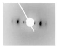
Figure 3: X-ray diffraction pattern showing the alignment of the lamellae parallel to the long axis of the capillary. (The capillary is very slightly tilted).
