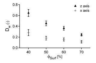
Figure 9: Variation of normalized water self-diffusion coefficients of aligned POM-doped lamellar phases with  $\phi_{Surf}$ , at constant  $\phi_{POM} = 3.5\%$ . The diffusion anisotropy can be clearly seen for all values of  $\phi_{Surf}$ ; moreover, it remains roughly constant.
