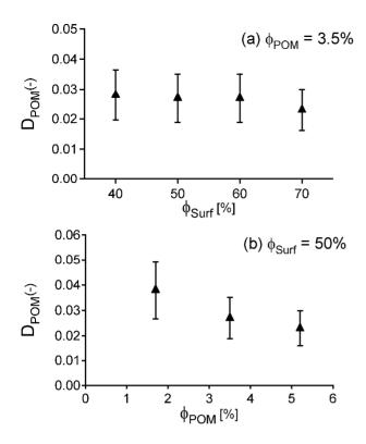
Figure 12: (a) Variation of normalized POM diffusion coefficients of aligned lamellar phases as a function of  $\phi_{Surf}$ , at constant  $\phi_{POM} = 3.5\%$ . (b) Variation of POM diffusion coefficients of aligned lamellar phases as a function of  $\phi_{POM}$ , at constant  $\phi_{Surf} = 50\%$ .
