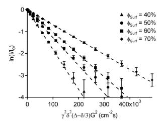
Figure 7: <sup>1</sup>H PGSE-NMR signal decays along the z-axis for samples with constant  $\phi_{POM} = 3.5\%$ and varying  $\phi_{Surf}$ . The decay is monoexponential in all cases. A linear fit using equation (1) gives the water self-diffusion coefficient perpendicular to the director of the L<sub>a</sub> phase.
