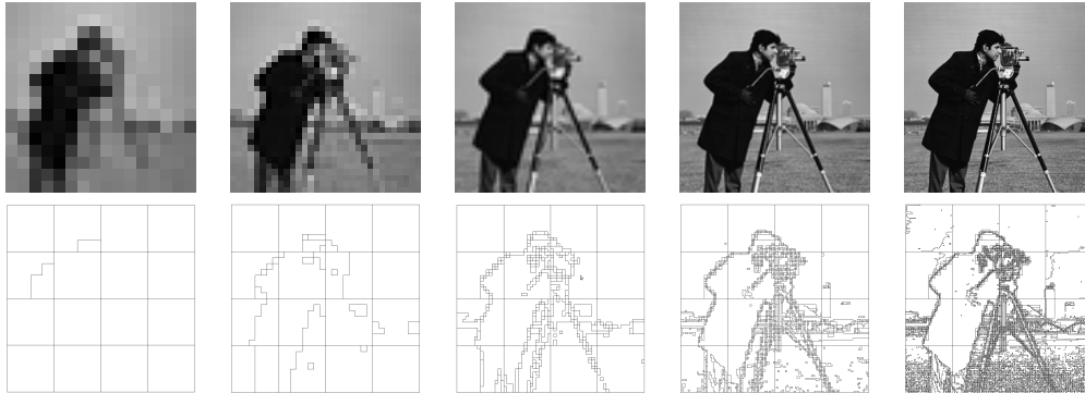
Figure 7: Extraction of a tiled top-down pyramid from a multi-resolution image based on the image Cameraman . First row displays the resolutions of the original image ( 16 \times 16 , 32 \times 32 , 64 \times 64 , 128 \times 128 , 256 \times 256 ). Second row presents the levels G^1 to G^5 of the tiled top-down pyramid (subdivision of 16 tiles/level).
