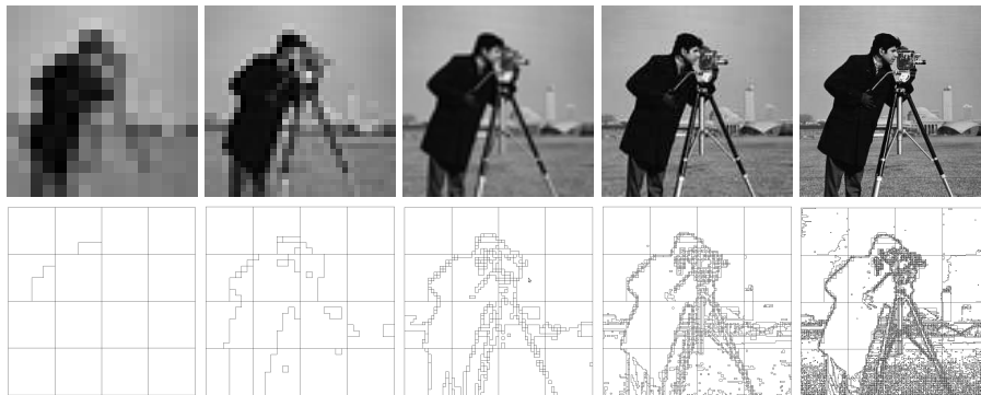
Fig. 7. Extraction of a tiled top-down pyramid from a multi-resolution image based on the image Cameraman . First row displays the resolutions of the original image ( 16 \times 16 , 32 \times 32 , 64 \times 64 , 128 \times 128 , 256 \times 256 ). Second row presents the levels G^1 to G^5 of the tiled top-down pyramid (subdivision of 16 tiles/level).
