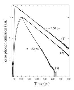
FIG. 8: Temporal decay at 6.5 K of the poly-3NPh2 zero phonon emission. (1) and (2): Zero phonon "broad" emission (II); (3) dynamics of the "narrow" emission (I). Curve (1) is obtained using a twelve times less dispersive grating (100 lines/mm). The pump power is always less than 50 nW.
