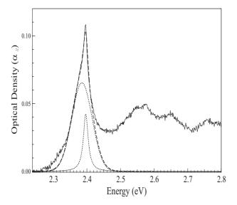
FIG. 2: Absorption spectrum, at 13 K, of a non irradiated crystal (solid line). The main exciton line is the sum of a Lorentzian contribution ( $\Gamma \sim 17$  meV) and a Gaussian contribution ( $\Gamma \sim 68$  meV, dotted line). Result of the fit: dashed line.
