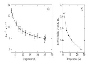
FIG. 9: Plot of  $\tau_{eff}^{-1}$  versus temperature for the narrow emission (I) at 2.401 eV. Two series of data are plotted (opened circles and squares). The solid line is the result of a fit  $\tau_{eff}^{-1} = \tau_{nrad}^{-1} + 1/\text{b}\sqrt{T}$ . b) Calculated quantum yield of emission deduced from the adjustment of  $\tau_{rad}$ .
