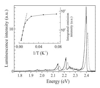
FIG. 6: : Emission of isolated chains of poly-3NPh2 at 8 K (solid line) and 55 K (dashed line). Inset: Arrhenius-like plot of the integrated emission intensity (solid line) and associated fit for T  $\succ$  60 K (dashes) giving an activation energy  $E_{act} \sim$ 22 meV
