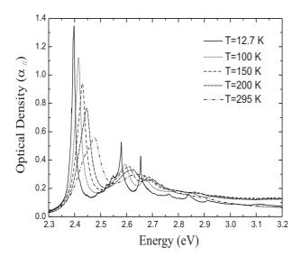
FIG. 3: Temperature dependence of the optical absorption,  $\alpha_{//}$  (incident electric field parallel to the **a**-axis), of isolated poly-3NPh2 chains in their host crystal ( $x_p \sim 4 \times 10^{-5}$ ). The sample thickness e~ 440  $\mu$ m leads to an absorption constant at the signal maximum,  $\alpha_{max} \sim 72 \text{ cm}^{-1}$  at 12.7 K.
