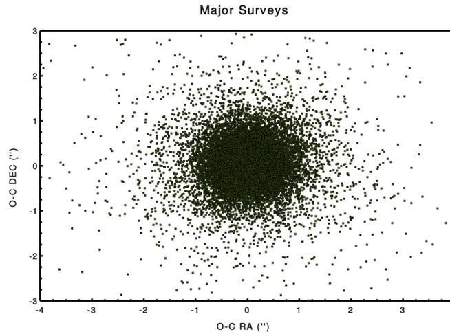
**Fig. 3.** Over 23,000 (o-c) residuals related with observations performed by all other surveys which observed in the past the same asteroids with EURONEAR. Comparing this plot with the one of Fig 2, one can observe that EURONEAR observations appear better confined around zero, and this fact is also supported by statistics.
