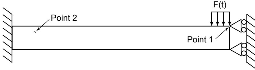
Figure 3. 2D-structure: boundary conditions, external forces, observation points 1 and 2
