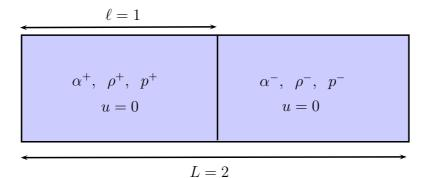
Figure 3. Sketch of the initial condition for the Sod shock tube test case.
