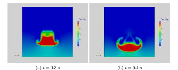
Figure 8. Water drop test case: falling and further deformation of the drop.
