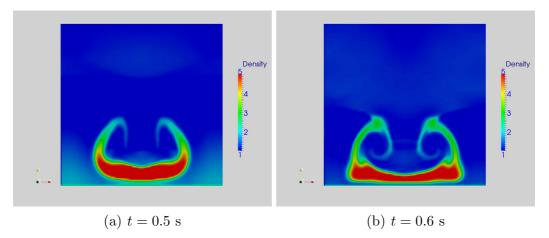
Figure 9. Water drop hitting the tank bottom.
