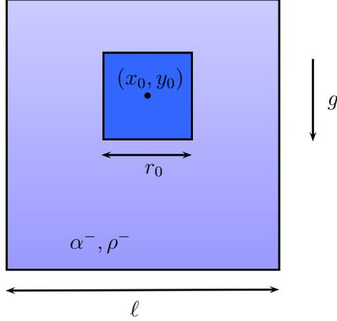
Figure 6. Sketch of the initial condition and computational domain geometry for the water drop test case. In our simulation we took the following values of geometrical parameters:  $\ell = 1.0$  (the domain is square),  $r_0 = 0.15$ ,  $x_0 = 0.5$  and  $y_0 = 0.7$ .
