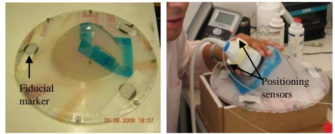
Fig. 5. Fiducial markers and positioning system for image matching
