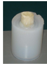
Figure 2. Child fibula sample embedded in an agar-gel shell
