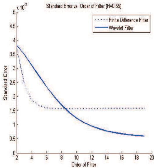
Fig. 3.: Comparison between the two types of filter.
