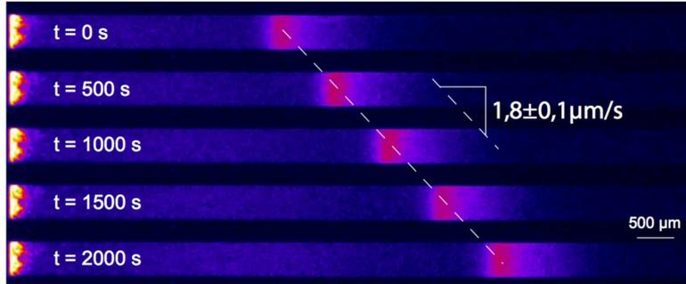
Figure 1: Experimental evidence for pulses of *Escherichia coli* traveling across a channel. The propagation speed is constant and the shape of the pulse front is remarkably well conserved. Observe that the profile is clearly asymmetric, being stiffer at the back of the front (see also Fig. 2). Cell division may not play a crucial role regarding the short time scale.
