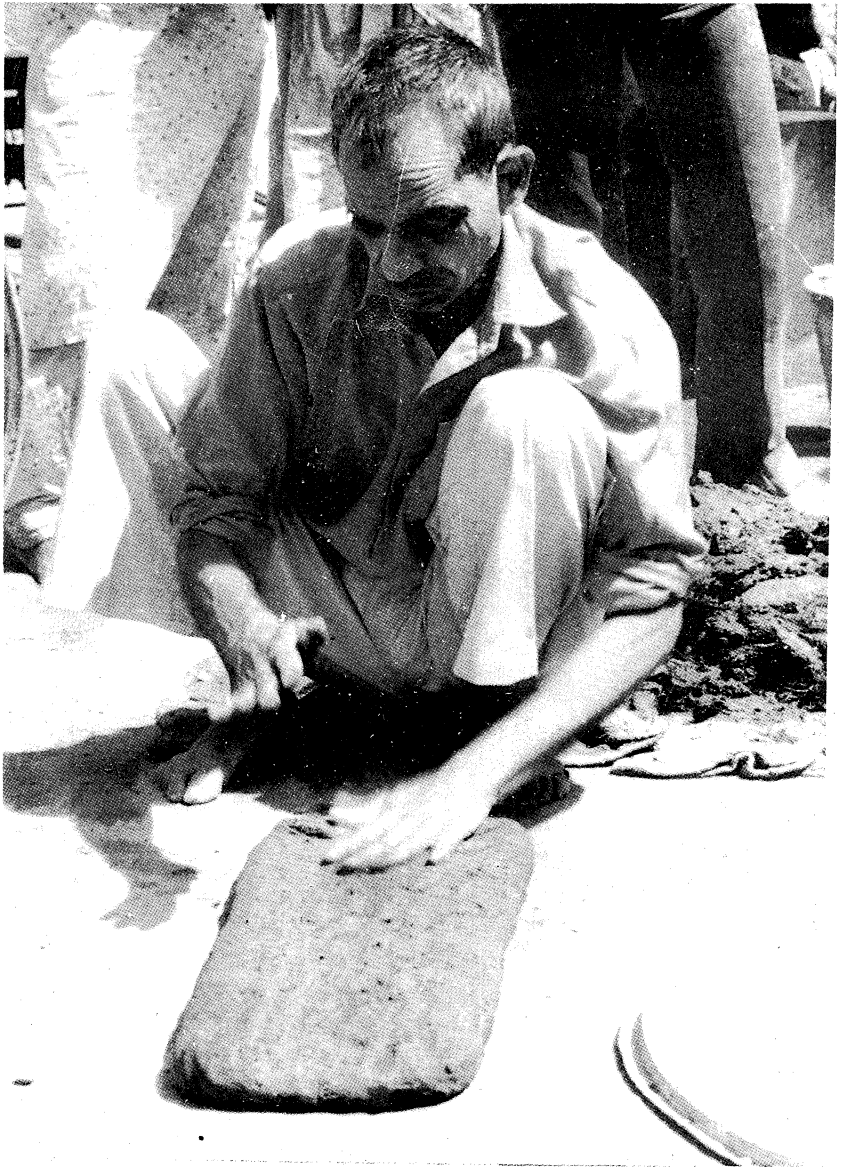
Plate 12: Manufacture of a clay slab aimed at constructing the lower part of a tandūr.
