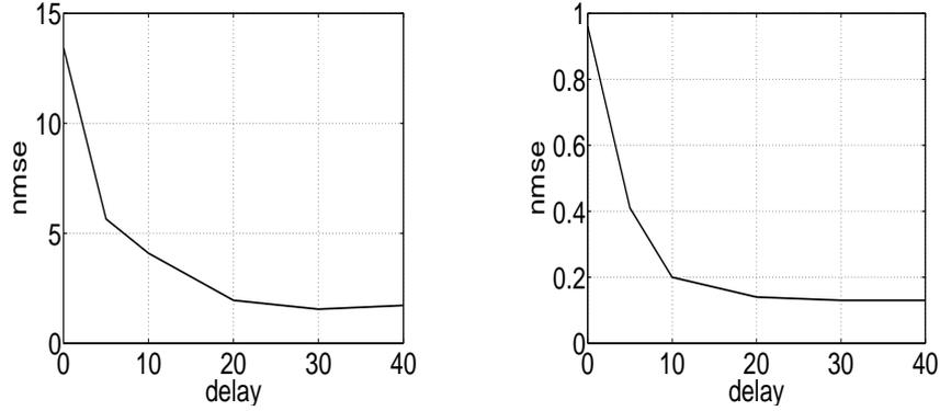
Figure 3: Validation normalized mean square error vs. time delays. The model is a neural network with 5 tanh neurons in the hidden layer and accepting  $A_p$  and  $\dot{\theta}$  as inputs. (left) Gear 2. (right) Gear 5.
