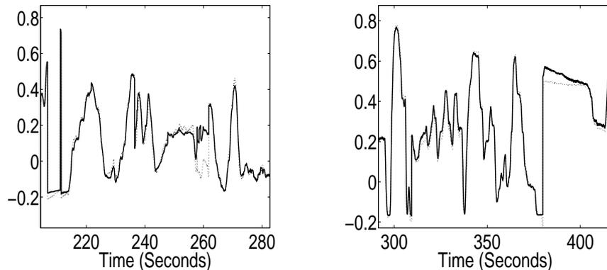
Figure 5: Examples of real (solid line) and estimated (dashed line) engine torques on validation set, best model (NN with 5 tanh neurons using  $A_p(t)$  and  $\dot{\theta}(t)$  as inputs). (left) Gear 2. (right) Gear 5.
