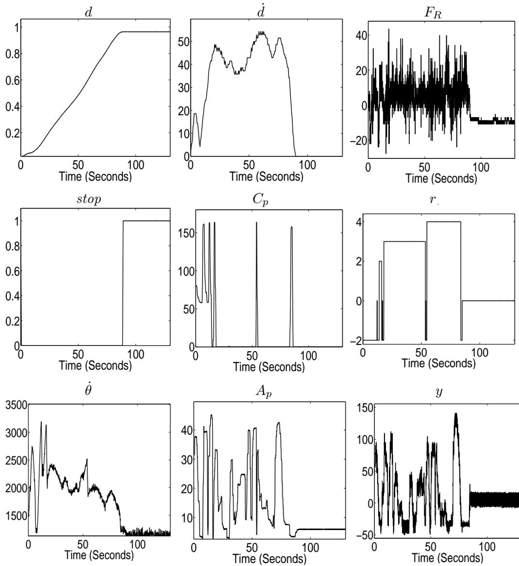
Figure 1: Examples of signals for a given data acquisition session.  $d(t)$ , distance covered by the vehicle,  $\dot{d}(t)$ , vehicle speed,  $F_R(t)$ , instantaneous load at the rear axle,  $stop(t)$ , binary indication of stopped vehicle,  $C_p(t)$ , clutch pedal position,  $r(t)$ , signal indicating which gear is engaged,  $\dot{\theta}(t)$ , engine speed,  $A_p(t)$ , accelerator pedal position,  $y(t)$ , net engine torque.
