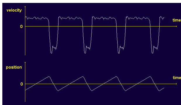
Figure 7: Velocity and position signals taken at the bowing point for our bowed string model. The bowing point is at a quarter of the string.
