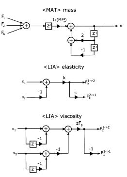
Fig. 4. Block diagrams of CA linear modules.
