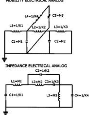
Fig. 5. Electrical analogous circuits of a CA model.
