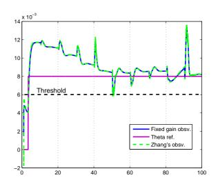
Fig. 5. 4mm fault estimation comparison.
