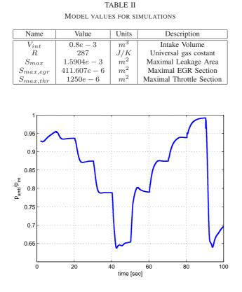
Fig. 3. Pressure ratio  $p_{amb}/p_{int}$  during a transient load at 1500 rpm.
