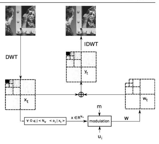
Exploitation of these weaknesses in the current watermarking algorithm is made by adding psychovisual masking in the wavelet domain. We use variable strength embedding [10]:
