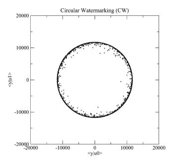
Fig. 9 Distribution of the projection of the marked signals over two carriers for CW,  $N_c = 2$
