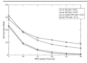
**Fig. 5** Robustness of the four proposed modulations against JPEG compression. For each modulation, the legend includes the standard deviation of the experiments
