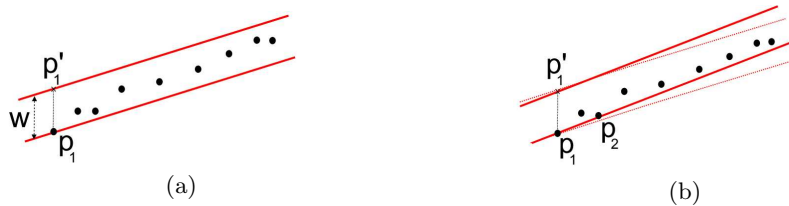
Fig. 1. A digital line that has one critical point p_1 (a), and its rotated digital line that has a second critical point p_2 (b).
