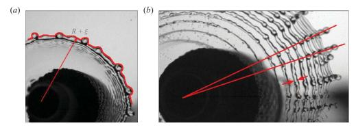
FIGURE 7. (Colour online) (a) Rim destabilization and the amplitude of corrugation,  $\xi$ . (b) Superimposed pictures of the sheet taken at constant time interval, showing sheet radius slowing, rim destabilization, rim diameter b constancy and wavenumber stretching.
