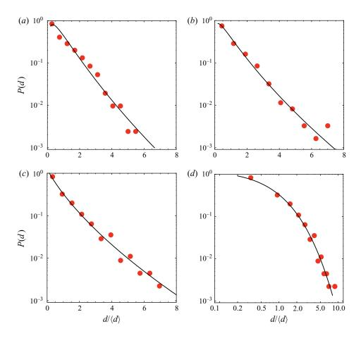
FIGURE 12. (Colour online) Global drop size distributions P(d) obtained for increasing Weber numbers, We = (a) 960, (b) 2870 and (c) 16930. Also shown is the distribution at (d) We = 16930 in log-log units. The solid line is a fit by (5.7) with n = 5 and m = 2, 1.5 and 1 (We = 960, 2870 and 16930 respectively).
