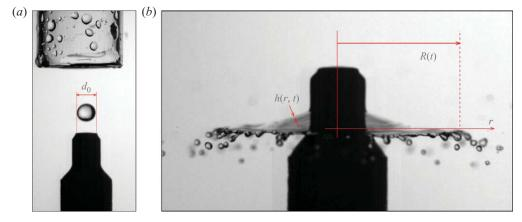
FIGURE 3. (Colour online) (a) A water drop just before it impacts the target of the same diameter  $2r_0 = d_0 = 6$  mm. Also visible is the confining tube used to prevent residual draughts from altering the drop trajectory. (b) Side view of the expanding sheet impaling on the impactor, 25/3000 s after the impact of the drop for We = 1800, and definitions of the sheet thickness h(r, t) and radius R(t). The velocity u(r, t) is the radial velocity in the sheet plane.
