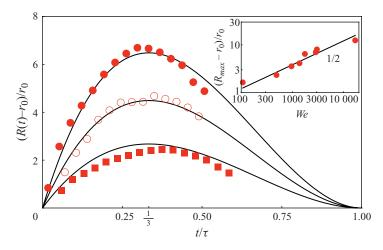
FIGURE 6. (Colour online) Sheet radius evolution as a function of dimensionless time  $t/\tau$  for three different impact Weber numbers, We = 489 ( $\blacksquare$ ), 1378 ( $\bigcirc$ ) and 2873 ( $\bullet$ ), superimposed with the trajectory expected from (3.16). The insert shows the dependence of the maximal sheet extension  $R_{max}$  on the Weber number. The line represents (3.18).
