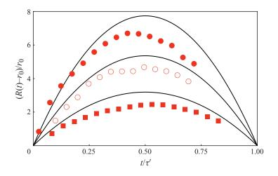
FIGURE 13. (Colour online) Sheet radius evolution as a function of dimensionless time  $t/\tau'$  for three different impact Weber numbers, We = 489 ( $\blacksquare$ ), 1378 ( $\bigcirc$ ) and 2873 ( $\bullet$ ), superimposed with the trajectory expected from (A 4). Compare with figure 6, where the fit by (3.16) is more satisfactory.
