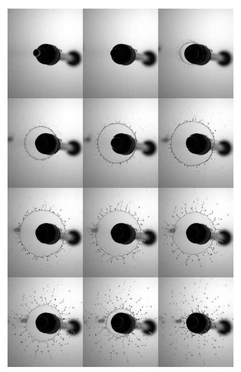
FIGURE 2. Sequence of events of the drop fragments' transformation following the drop (visible in the first image) impact on a target of the same diameter  $d_0 = 6$  mm. The liquid is ethanol, and the Weber number is We = 1200. The time interval between the pictures is 1/500 s.
