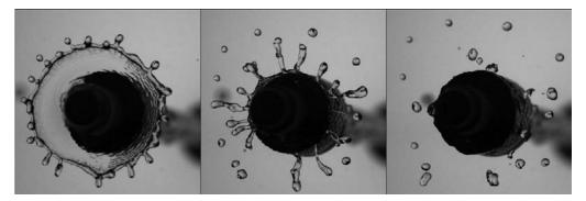
FIGURE 9. Construction of the elementary drop size distribution from the breakup of similar ligaments. The first image is a snapshot taken close to the maximal sheet extension 1/100 s after drop impact. The time interval between the images is 1/100 s; We = 490.
