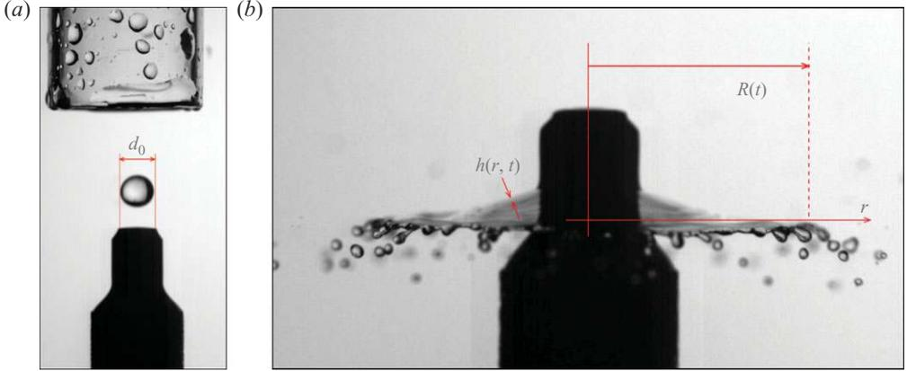
FIGURE 3. (Colour online) (a) A water drop just before it impacts the target of the same diameter  $2r_0 = d_0 = 6$  mm. Also visible is the confining tube used to prevent residual draughts from altering the drop trajectory. (b) Side view of the expanding sheet impaling on the impactor,  $25/3000$  s after the impact of the drop for  $We = 1800$ , and definitions of the sheet thickness  $h(r, t)$  and radius  $R(t)$ . The velocity  $u(r, t)$  is the radial velocity in the sheet plane.
