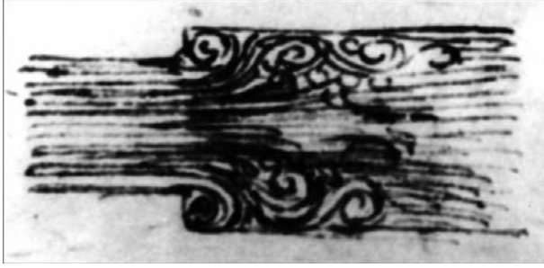
FIGURE 14. An abrupt expansion from a section A_1 with velocity u_1 to a section A_2 with velocity u_2 accompanied by turbulence and vortices, as imagined by Leonardo Da Vinci (1508).
