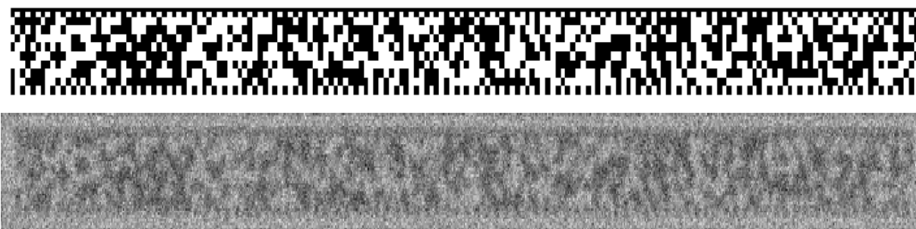
Fig. 7. A 2D Alphacode chain of character (60 data characters and 30 redundant characters) with a dot of 4x4 pixels and a blur matrix of 5x5. This image is corrupted with a noise with E_p/N_0 = 0 dB, where E_p is the mean energy received by one dot and N_0 the spectral density of the noise.
