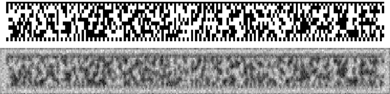
Fig. 8. A 2D Alphacode chain of character (60 data characters and 30 redundant characters) with a dot of 2x2 pixels and a blur matrix of 3x3. This image is corrupted with a noise with E_p/N_0 = 9 dB, where E_p is the mean energy received by one dot and N_0 the spectral density of the noise.
