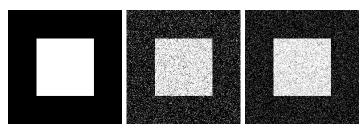
Fig. 7. Original scene (with two classes: the white square and the background) and two noisy observations, simulating two information sources, and defining  $m_0^1(C_1)$  and  $m_0^2(C_1)$ .
