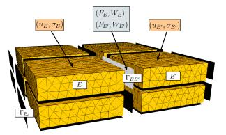
Figure 4: Substructuring of the laminated composite structure
