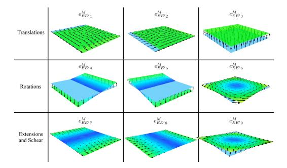
Figure 5: The linear macro basis for a plane interface
