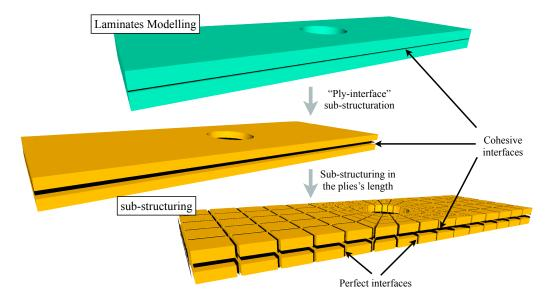
Figure 3: Substructuring of the laminated composite structure
