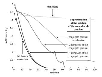
Figure 18: LaTIn convergence curves for different numbers of macro iterations
