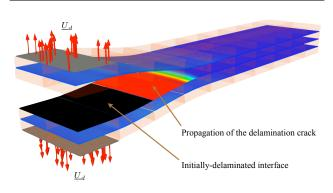
Figure 7: Four-ply DCB test case
