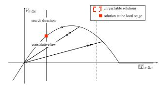
Figure 9: Using infinite value for Search direction parameter  $k^+$
