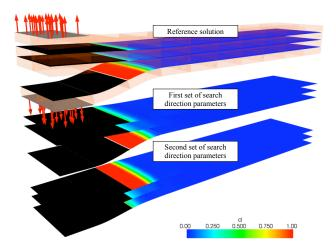
Figure 10: Converged solutions reached by the LaTIn algorithm using different sets of search direction parameters
