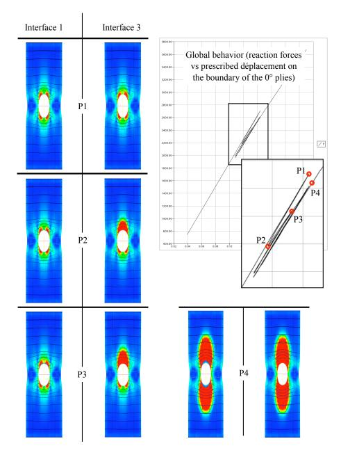
Figure 23: Behavior of the holed plate under traction
