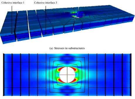
(b) Damage in Cohesive interface 1
