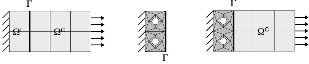
**Fig. 3** Global, local and reference FE models (darker elements are elastic-plastic)
